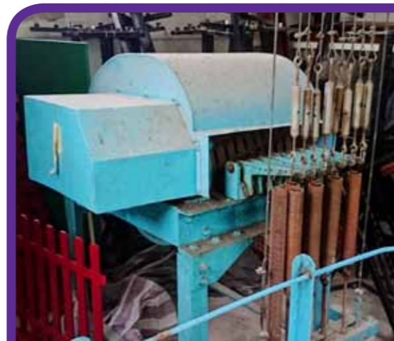
PHOTO 4 — Electro-mechanical system for ringing the chime. Works on the same principal as a "musical box cylinder". Originally installed in 1953 - now obsolete
